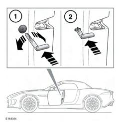
In the event of the battery discharging or a fault with the Keyless locking system, the doors must be locked manually.
