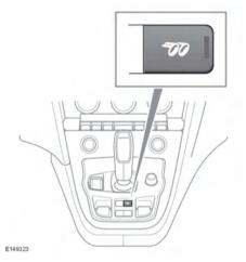
For vehicles with Active exhaust, this system will operate valves in the exhaust to produce a richer and louder noise to enhance the driving experience.
