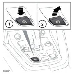
With the ignition switched on, depress the brake pedal and press down on the EPB switch (1). This will release the parking brake.
