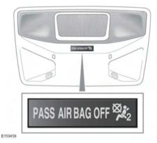
A warning lamp in the roof console will illuminate if Passenger Airbag Off setting is selected.
