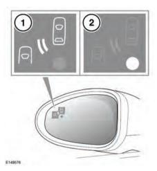
If an object is identified by the system as being an overtaking vehicle/object, an **amber** warning icon (1) illuminates in the relevant exterior mirror, to alert the driver that there is a potential hazard in the vehicle's blind spot and therefore, that a lane change might be dangerous.
