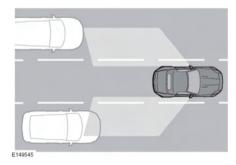
The Blind Spot Monitor (BSM) system monitors a zone that covers the area adjacent to the vehicle, that is not easily visible by the driver and is designed to identify any object overtaking the vehicle. The system uses a radar on each side of the vehicle to identify any
