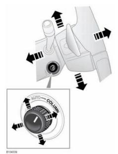
The steering wheel can be adjusted for tilt and reach as follows:
