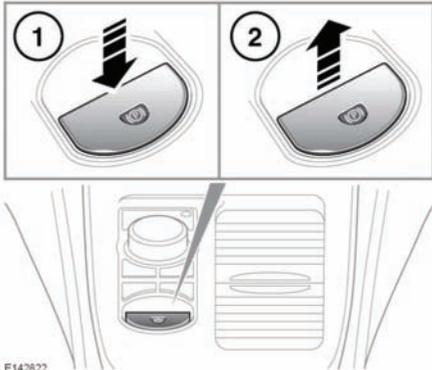
With the ignition turned on, press the brake pedal and press down on the EPB switch (1). This will release the electronic parking brake.
