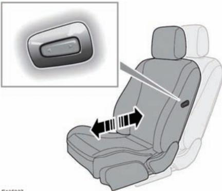
When fitted the driver can adjust the position of the front passenger seat, press for forward or rearward adjustment.
