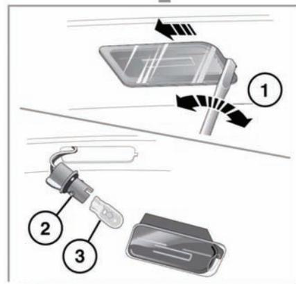
1. Insert a small flat-bladed screwdriver into the indent as shown and carefully lever out the side of the lamp unit and remove.
