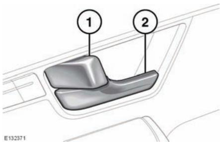
1. Press the locking lever to lock the door, pull the lever to unlock the door. Operating the locking lever on either front door will lock or unlock all closed doors.
