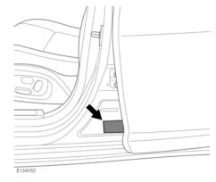
The recommended tyre pressures are listed on a label located in the left side front door opening.
