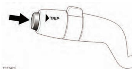
Press the **TRIP** button on the end of the left column stalk repeatedly to display the trip data in the following order:
