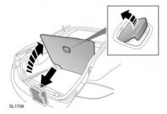
Your vehicle may not be equipped with a spare tyre. If this is the case, in its place in the rear underfloor storage compartment, you will find a tyre repair kit (except where run-flat tyres are fitted). The tyre repair kit can be used to repair **one** tyre and it is essential that you read the following guide before attempting to repair a tyre.
