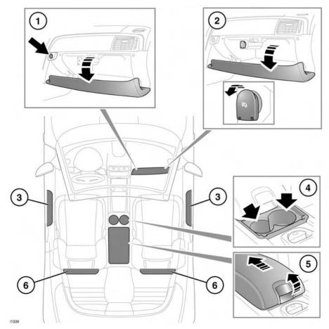
1. Glove box: Open using the glove box release (arrowed).
