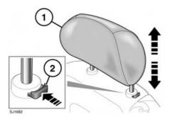
To raise, pull the restraint (1) upwards, it will click and lock in position.
