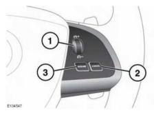
The cruise (speed) control system can be used by the driver to maintain a selected vehicle speed above 30 km/h (18 mph).
