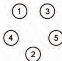
Using the wheel nut wrench, lightly tighten the wheel nuts alternately using the sequence shown in the illustration.
