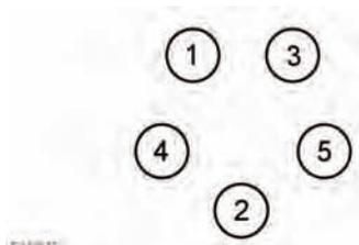
Using the wheel nut wrench, lightly tighten the wheel nuts alternately using the sequence shown in the illustration.
