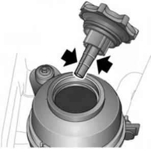
1. Clean the filler cap before removing to prevent dirt from entering the reservoir, see **145, ENGINE COMPARTMENT OVERVIEW**.
