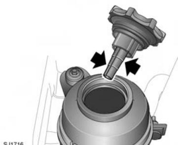
1. Clean the filler cap before removing to prevent dirt from entering the reservoir, see **145, ENGINE COMPARTMENT OVERVIEW**.
