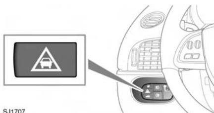
Press the button to switch Forward alert on or off.
