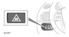
Press the button to switch Forward alert on or off.
