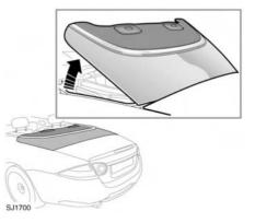
• Fully open the tonneau panel. It will self-support when fully open.
