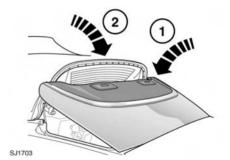
Supporting the tension bow, lower the tonneau panel (1). Then lower the tension bow (2) onto the tonneau panel.
