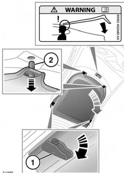
**To remove the luggage cover:** Release the two latches (1) and slide the cover downwards and forwards, so that the two rear locating pegs (2) are disengaged. This will allow the cover to be removed.
