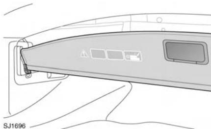
When the convertible roof is closed, the normal position for the luggage separator is in the retracted position, with the partition positioned vertically (as shown).
