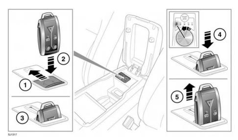
If the Smart Key fails to operate, **Smart Key Not Found- Refer to Handbook** is displayed in the message centre. To start the engine it will be necessary to dock the Smart Key, as follows:
