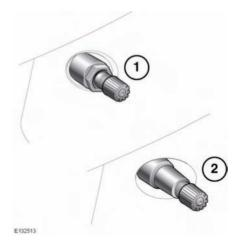
Wheels fitted with a TPM system can be visually identified by the external metal lock nut and valve (1). All Jaguar non-TPM system wheels have a rubber valve fitted (2).
