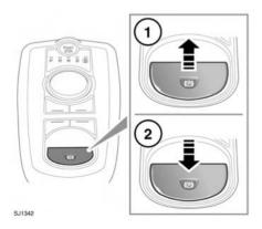
The switch which operates the parking brake is mounted on the centre console to the rear of the gear selector.
