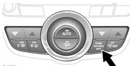
The airbag indicator, on the centre console, is associated with the deployment conditions for front seat passenger airbags only.
