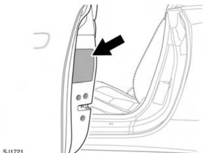
The recommended tyre pressures are listed on a label located on the end of the left-hand side door.
