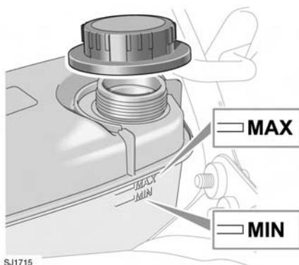
Ensure the coolant level is maintained between the level indicator marks, as shown in the illustration.
