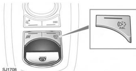
The **ASL** button allows the driver to select between cruise control and the automatic speed limiter. The ASL can be set to any speed between 30 km/h (18 mph) and 240 km/h (150 mph).
