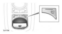
The **ASL** button allows the driver to select between cruise control and the automatic speed limiter. The ASL can be set to any speed between 30 km/h (18 mph) and 240 km/h (150 mph).
