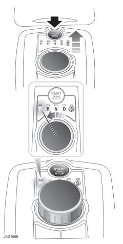
The JaguarDrive selector elevates out of the centre console when the engine is started, in readiness for gear selection. Press the brake pedal, then rotate the control to select the chosen gear (P, R, N or D). To select S (Sport), rotate the control to D, then press down on the control and rotate to select S.
