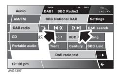
Briefly touch one of the channel seek buttons to select the next available digital channel. The seek up button selects the next channel, the seek down button selects the previous channel.
