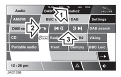
If subchannels are available under the current channel, the subchannel arrow icon (1) is displayed at the top of the touch-screen and the Subchannel button is enabled.
