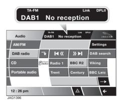
If the digital radio signal is lost or the system takes time to tune in to a channel, then the display screen will show the message **No reception**.
