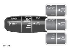
Three settings on the rotary collar set the time that the headlamps will remain on after the driver's door has closed:
