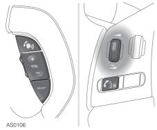
Once a phone is docked in the cradle, you must tell the system to use the phone in the cradle by pressing the 'Telephone/Voice recognition' switch until an audible response is heard.
