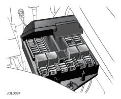
This fuse box is located in the luggage compartment, situated behind the battery.
