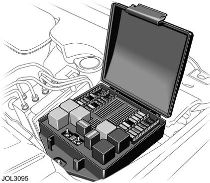
The fuse box is located in the engine compartment on the right-hand side adjacent to the windscreen wash reservoir.
