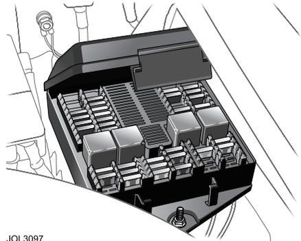
This fuse box is located in the trunk, situated behind the battery.
