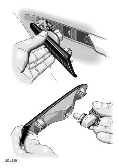
To remove the light unit from the front wing, push the lens towards the front of the vehicle to compress the spring clip and then pull the rear outwards to remove the complete unit.
