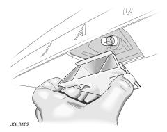
Press the two lens clips inwards and remove the lens from the vehicle.
