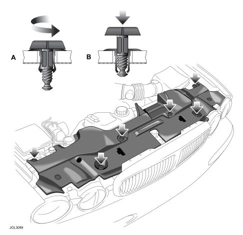
To gain access to the headlight units, the top cover must be removed.
