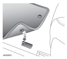
The driver's floor mat is correctly must be correctly positioned and secured under the tongues on the retention posts (only one post shown). Ensure that the mat does not interfere with the operation of the accelerator or brake pedal.
