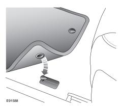
The driver's floor mat must be correctly positioned and secured under the tongues on the retention posts (only one post shown). Ensure that the mat does not interfere with the operation of the accelerator or brake pedal.
