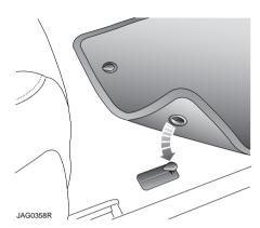
Ensure that the driver's floor mat is correctly positioned and secured under the tongues on the retention posts (only one post shown), so that the mat does not interfere with the operation of the accelerator or brake pedal.
