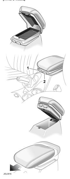
The sliding armrest is hinged at the rear and has two release buttons located on the front of the armrest.
