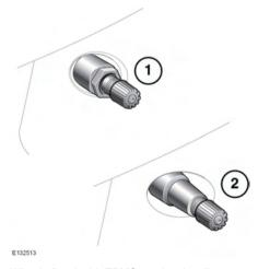
Wheels fitted with TPMS can be visually identified by the external metal lock nut and
