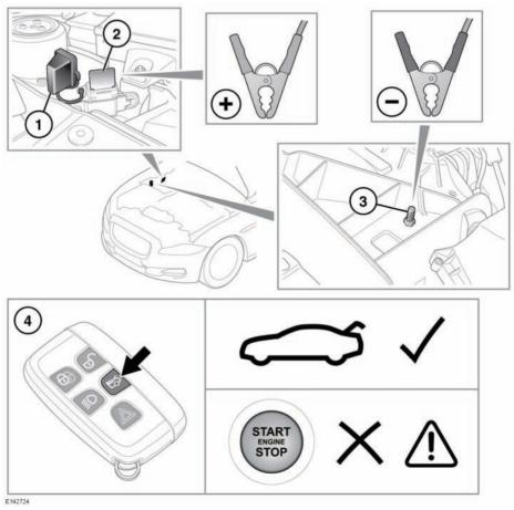
With the bonnet open and the engine cover removed (see **187**, **FUSE BOX LOCATIONS**), connect jump lead cables to a suitable 12v supply. Then:-
