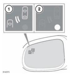
If an object is identified by the system as being an overtaking vehicle/object, an **amber** warning icon (1) illuminates in the relevant exterior mirror, to alert the driver that there is a potential hazard in the vehicle's blind spot and therefore, that a lane change might be dangerous.
