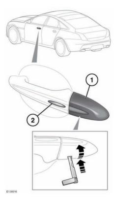
Insert the key blade into the slot in the door lock cover (1).
