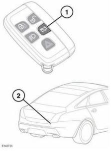
The luggage compartment can be opened using the appropriate button on the Smart Key (1), or via keyless entry. It can also be opened using the exterior release (2), provided the doors are unlocked and the gear selector is in Park (P).
