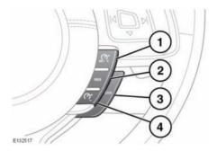
SET+: Press to set the speed or to increase the set speed. The cruise control warning lamp will illuminate to confirm cruise control is operational (see 53, CRUISE CONTROL (GREEN)).
