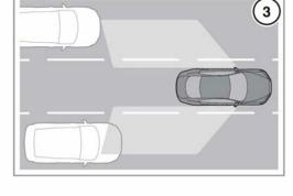
The Blind Spot Monitor (BSM) system monitors a zone that covers the area adjacent to the vehicle, that is not easily visible by the driver and is designed to identify any object overtaking the vehicle (3). The system uses a radar on each side of the vehicle to identify any overtaking vehicle/object within the blind spot area of the vehicle, while disregarding other objects which may be stationary or travelling in the opposite direction, etc.
