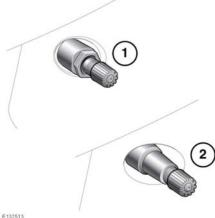
Wheels fitted with TPMS can be visually identified by the external metal lock nut and valve (1). All Jaguar non-TPMS wheels have a rubber valve fitted (2).
