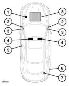
1. Left-hand front suspension tower - Air conditioning label.
