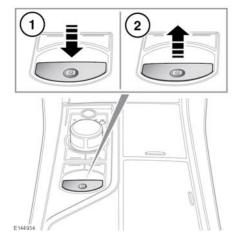
With the ignition turned on, press the brake pedal and press down on the EPB switch (1). This will release the electronic parking brake.
